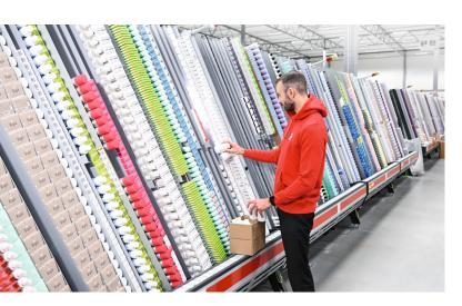
The A-Frame from SSI SCHAEFER performs complex order consolidations automatically, reliably, and as quickly as possible. It is particularly suitable for picking small packaging units without errors. Thanks to a sophisticated system with both straight and inclined product channels, the throughput of fast and medium movers is increased dramatically.
