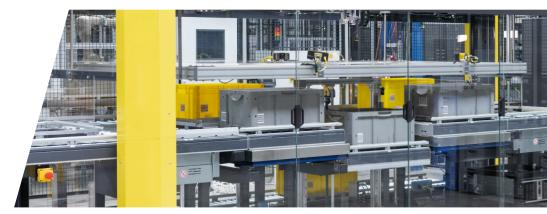
SSI Piece Picking enables fully automated piece picking. It is used where individual pieces in the small parts area have to be picked and highest precision is required. This versatile solution, which includes a dedicated smart software, boasts advanced functions such as pick-and-place, object recognition using artificial intelligence (AI), a patented gripping point determination, and extremely gentle product handling.
