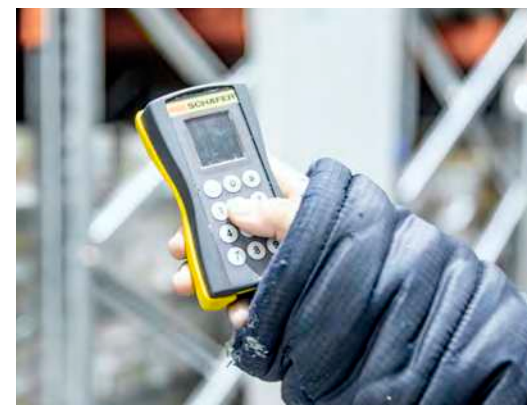
Handheld controller to select the aisle required for work
