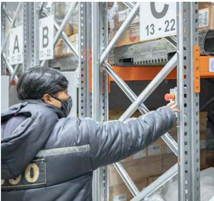
Equipped with both manual stop switch and safety laser device
