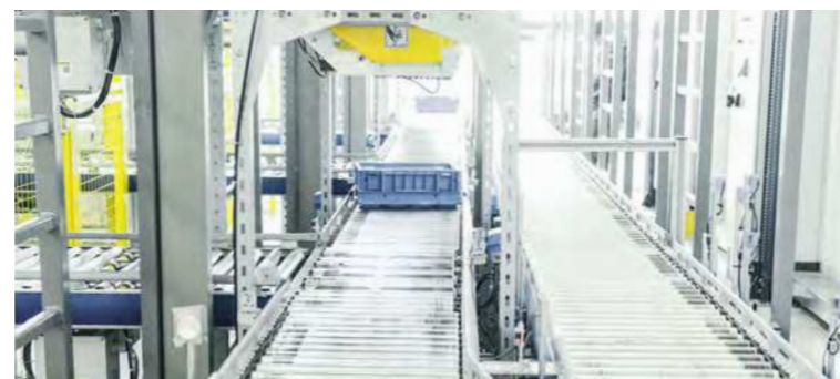
Components retrieval from pallets in VNA or bins in SSI Miniload
