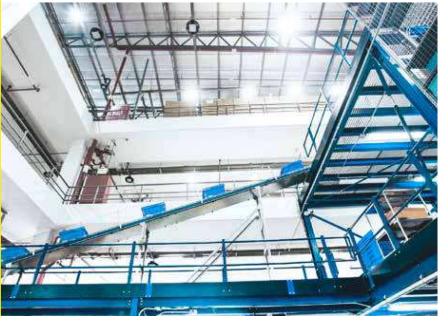
Carton and bin conveying system for economical transport
