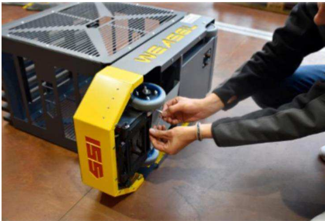
Fig. 11 | Removal of transportation fixtures
