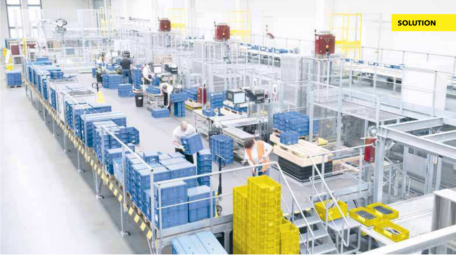
The transfer carriage delivers source pallets that are not delivered in system totes to the manual repacking stations
