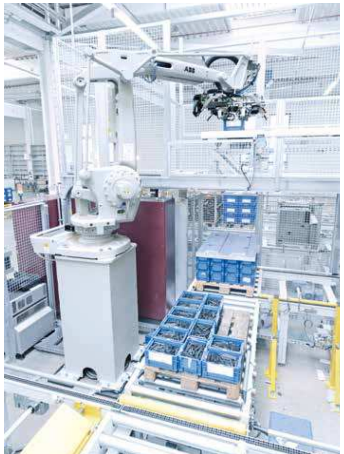
The robot is equipped with a special gripper finger system for transferring.
