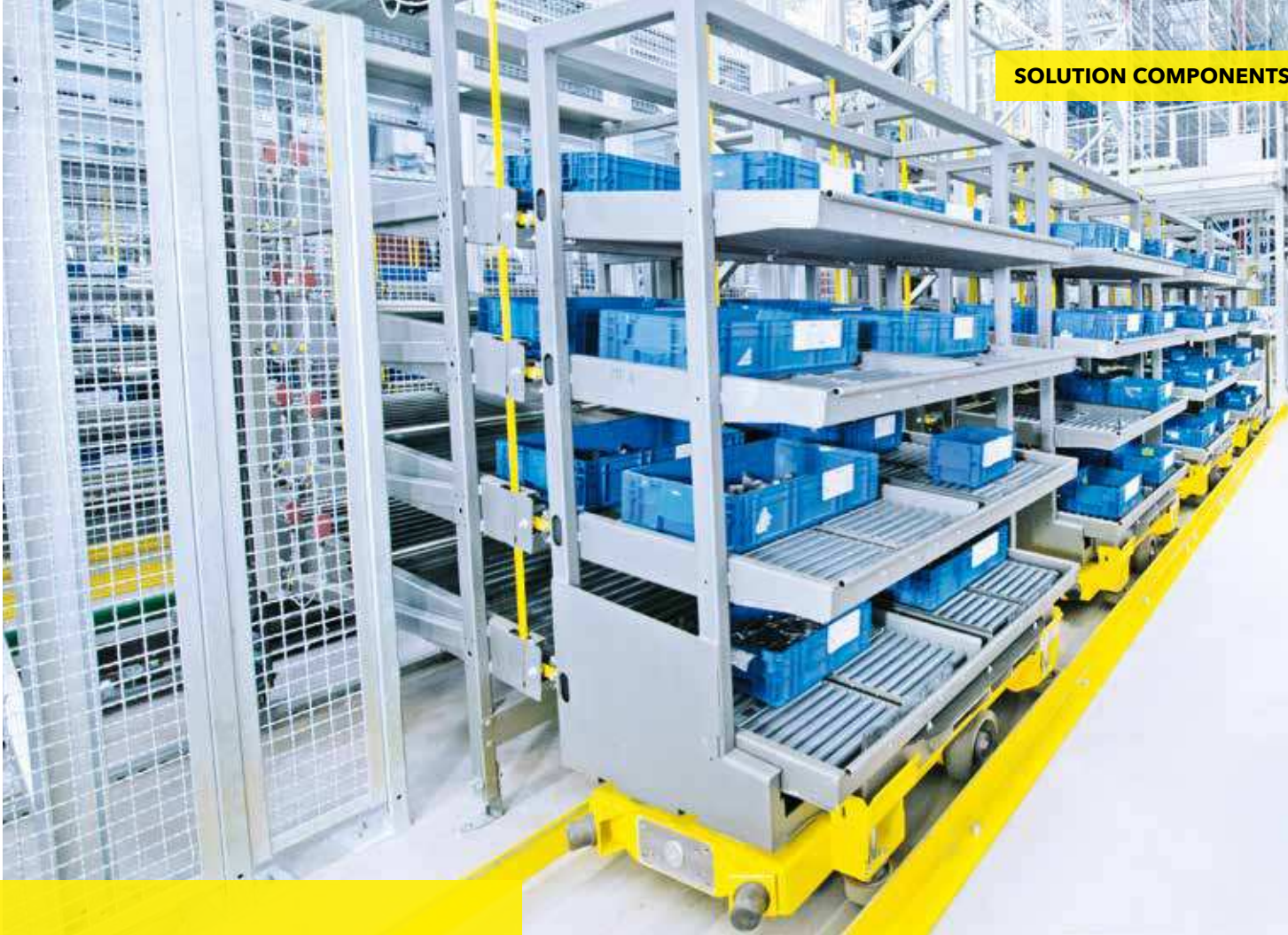
Bins are released once the trolley train reaches the loading position.
