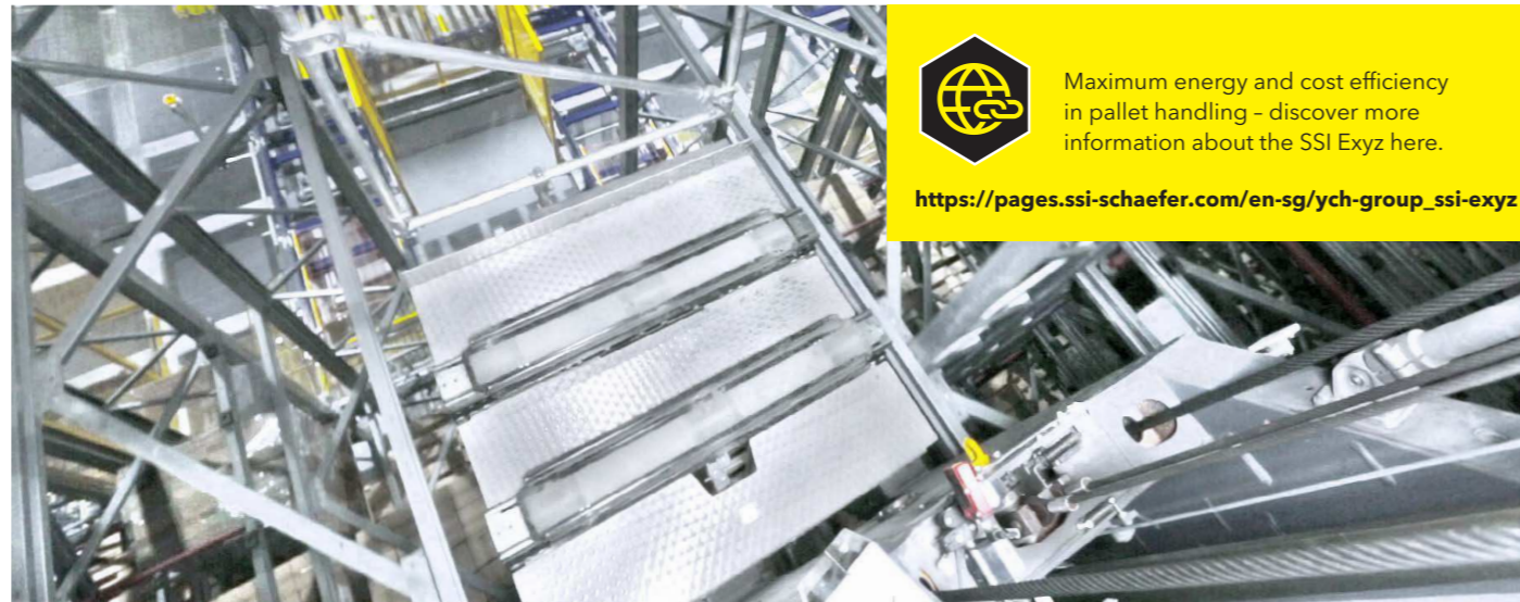
Single-mast, double-deep automated storage-retrieval machines
