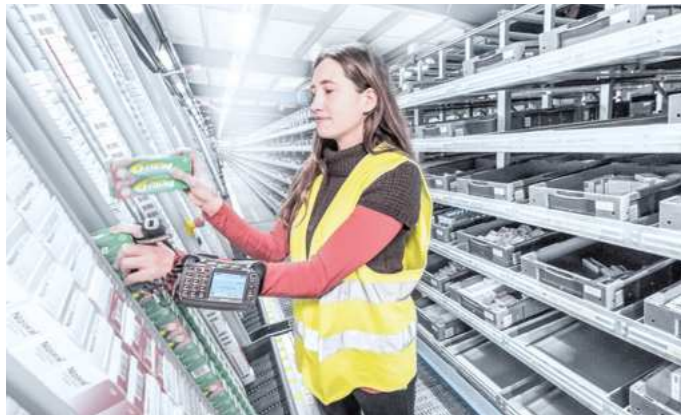
A-Frame replenishment from flow racks
