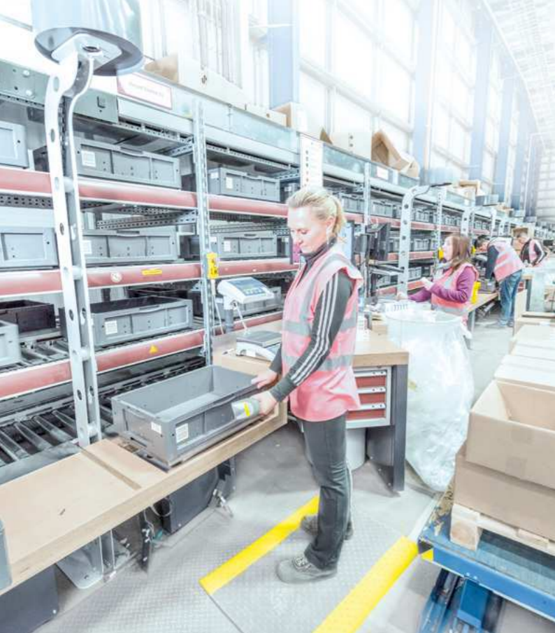
Repacking of delivered goods at ergonomically optimized goods-in workstations
