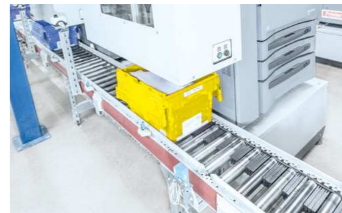
Automatic delivery note insertion
